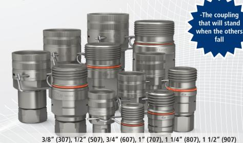
TLX is a Flat-Face twist lock coupling for the toughest applications in the construction and demolition segment. This super-duty quick connect coupling is designed to work with the highest surge flows and the toughest pressure impulses. TLX is made from high alloy steels with Zinc-Nickel surface treatment for a long life in the harshest conditions. The Series is available in sizes from 3/8" to 1 ½" to cover most applications.
