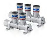
The CEJN Multi-Link lets you connect as many outlets as you need at each distribution point to form an efficient air distribution system. The outlets can be positioned at different angles and still assure an unobstructed and high air flow. The units can be supplied with compressed air from either end and come in 2,3,4 or 5 outlet versions. Eliminates the need for elbows, tees, unions and nipples that can result in jumbled piping configurations.
