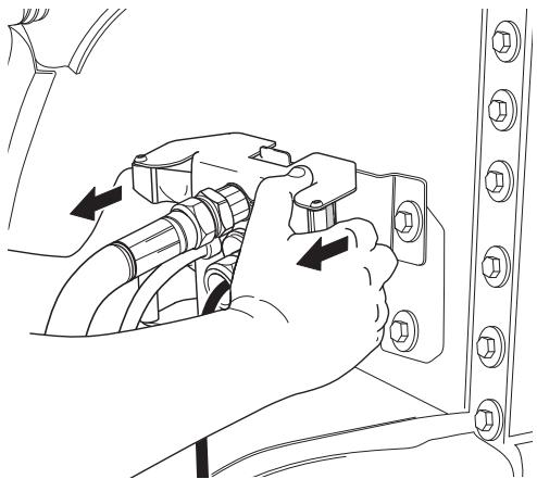
Attach the hose plate in its parked position on the ramp by PUSHING it INTO the ramp plate. This is best achieved by pressing the plates together with the fingers while holding onto the handles of the ramp plate.
