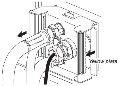
PULL OUT the plate from the bus using the black handles.
