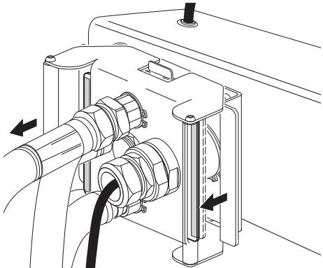
PULL OUT the hose plate from the ramp using the black handles.
