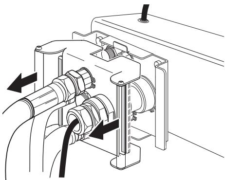
Attach the hose plate to the bus by guiding the pin into the centre hole and PUSHING the hose plate IN. This is best achieved by pressing the plates together with the fingers while holding onto the handles of the bus plate.
