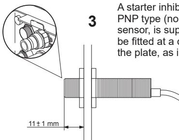
**3** A starter inhibitor sensor, which is a PNP type (normally closed) inductive sensor, is supplied separately and must be fitted at a distance of  $11\pm 1$  mm from the plate, as illustrated in the diagram.
