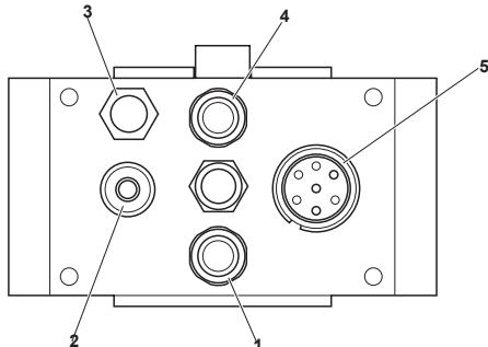
**1** Return fluid exits from the BLUE colour-coded nipple marked OUT. The nipple (the male connector) has an inside G 1/2" thread which fits the 16 mm (5/8") or 19 mm (3/4") hose adapters supplied.
